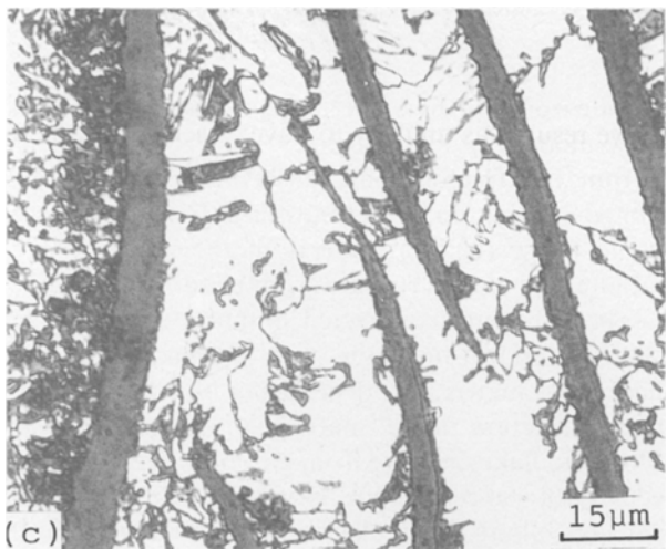
Figure 5 Optical micrographs of cast irons austenitized 20 sec at 950°C. (a) spheroidal graphite iron (b) compacted graphite iron (c) flake graphite iron.
